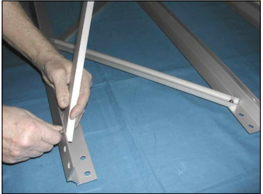
First stray to put on the next side of the left corner leg. The M6x16 screw is used here as it is a two material connection.
