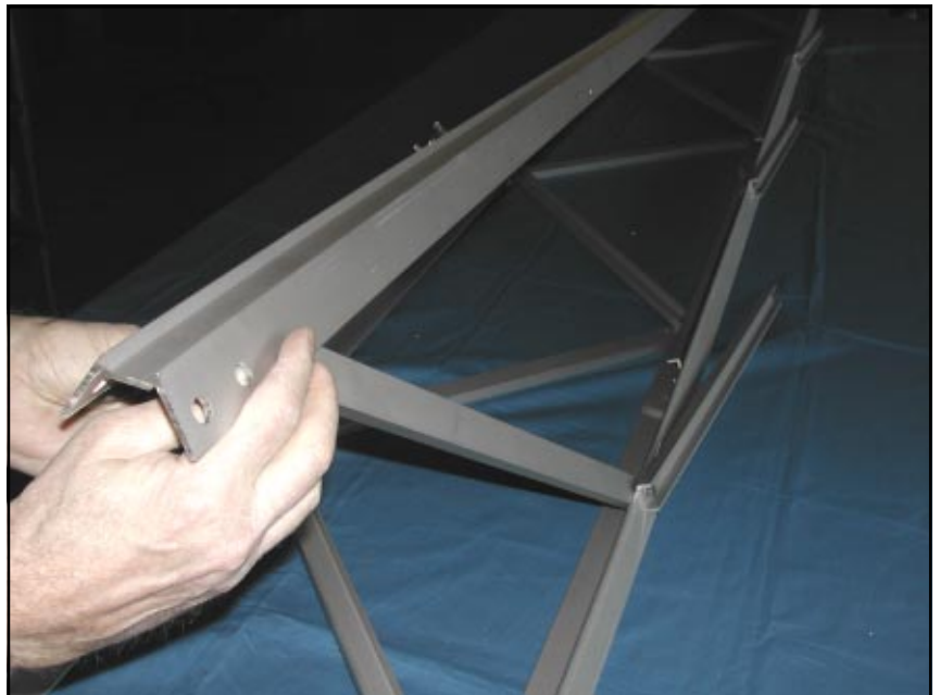
Third side of construction being attached by the first stray on its side to the third corner leg. Here a two material connection thus an M6x16 with washers and nut
