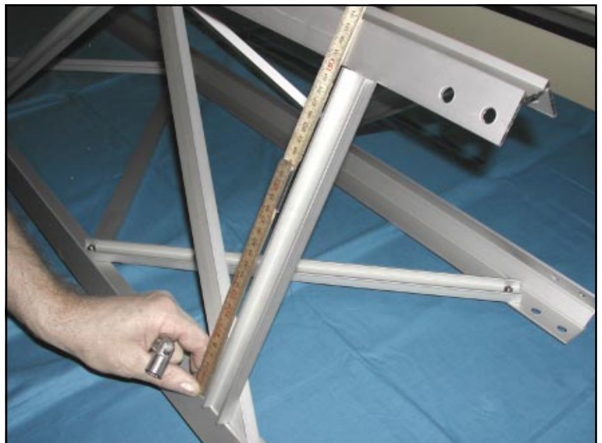
The 303 mm distance does not have to be mounted in any way. It stays nicely in position while in use. Do an extra measure to be sure of the distance.
