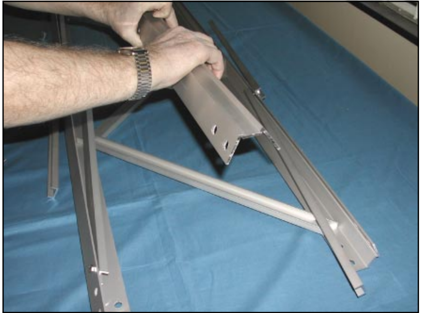
The third corner leg brought into position to be connected to the strays recently folded back in stand-by position
