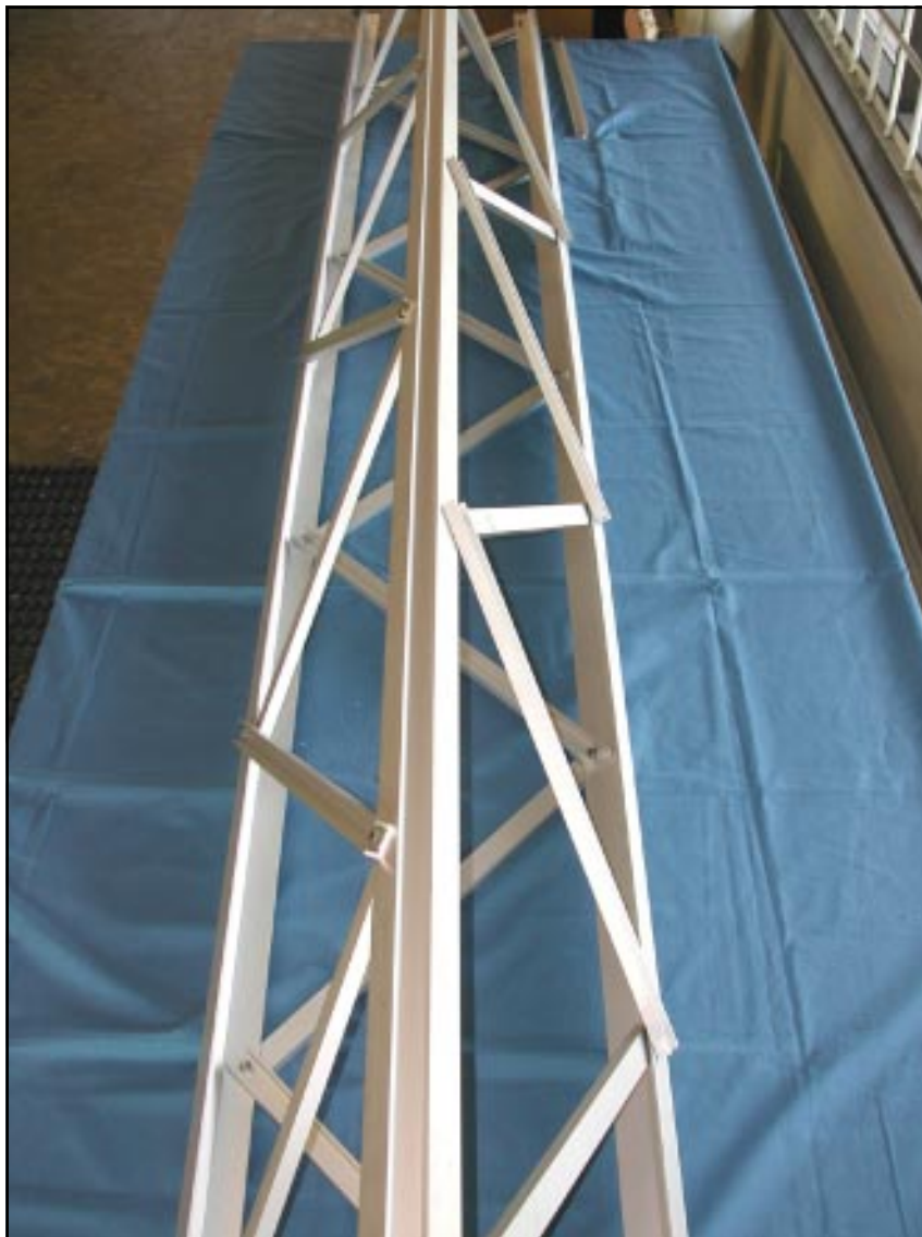
Neat looking assembled section. Still not ready to go into the tower as all connections need to be tightened securely
