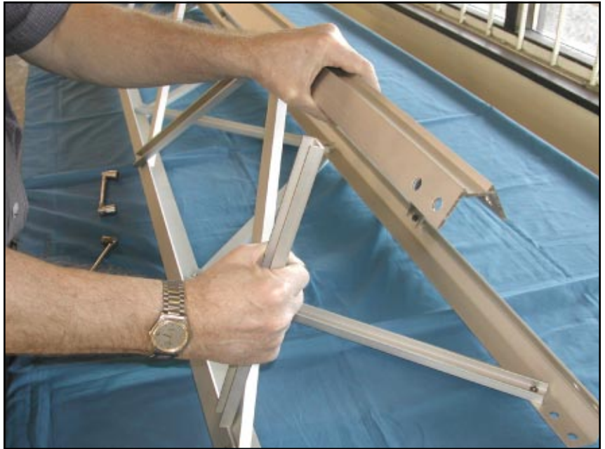
The 303 millimetre special distance profile supplied in the kit is the helper to achieve correct spacing between the corner legs
